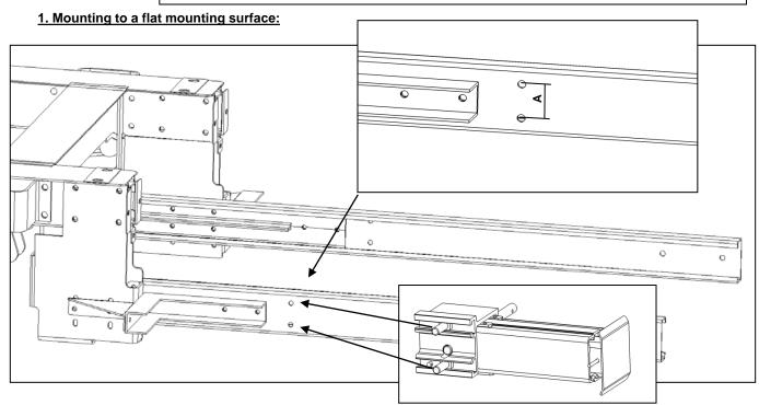
If there are no holes in the frame extension, they have to be drilled.
